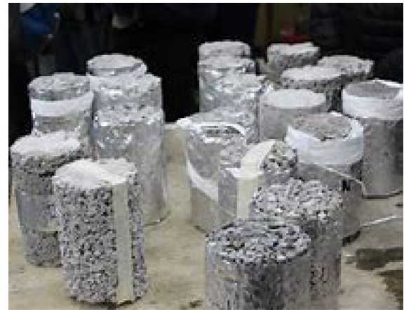
Fig. 3. (a) Porous Concrete cube; (b) Pervious concrete cylinders.
